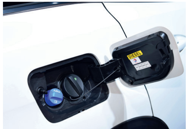
Opening designed for AdBlue® refills in the fuel tank flap - rolled out on all Group vehicles.
